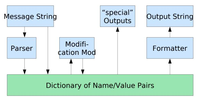
Arriving messages are run either through parsers or stored directly by the input module in a dictionary of name/value pairs, which is the actual internal rsyslog
