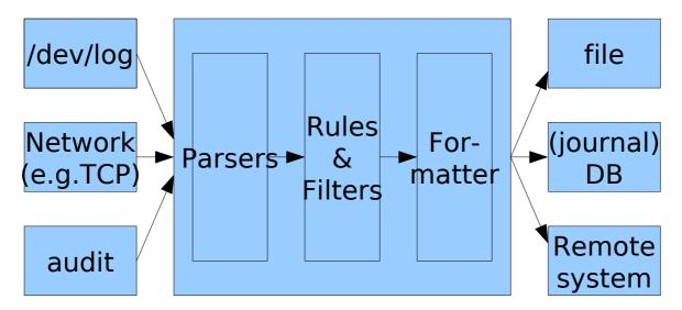
On the left-hand side are input modules. These gather data from various sources, like files, the log socket or network protocols like syslog. Each of these modules can be thought of as an individual project (and actually is) and each can by dynamically loaded.
